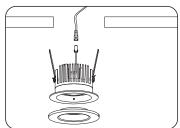
Feed cables thorough and make the electoral connections to the led driver according to relevant regulations in your territory.
