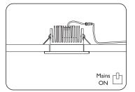
Turn mains electricity back on and test to see if the product is functioning correctly
