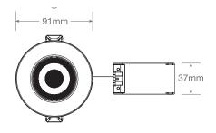
Cutout: Ø58 -75 mm Overall Diameter: Ø91 mm Overall Depth: 72 mm
