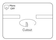
Choose the location of your new downlight, giving consideration to joists, water pipes, wiring or any other obstacles that may hamper installation. Please also ensure you have adequate ventilation and/or ceiling clearance in the relevant voids.
