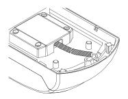
lect the desired output using the CCT switch. Close the connection cover
